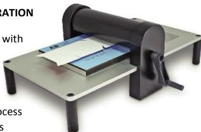
The crease to be tested can be cut with a single process therefore eliminating errors associated with traditional crease sample preparation (usually a 3 step process). Multiple test pieces can be cut from the same sample saving valuable test time. Hanatek offers custom cutting dies to suit most packaging applications, e.g. friction, tensile, grammage, rub / abrasion.
